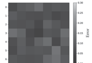
Fig.2: Error distribution of reverberation time at 1 kHz
