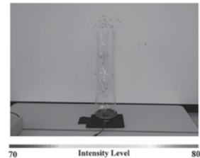
Fig. 2: Measured sound flow of an air column resonating at its 3rd harmonic. The antinode can be seen further away from its opening due to end correction.
