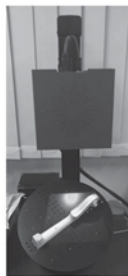
Fig.2: 3D scanner (Gom core 200 5M)
