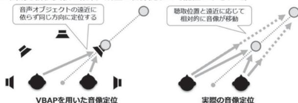
Fig. 1. Difference of a sound localization between an actual sound source and a sound image reproduced by VBAP (left: VBAP, right: Actual)
