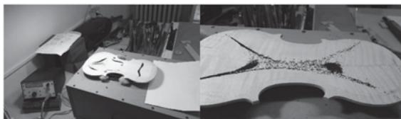
Fig.1 Vibration mode by Chladni method (right: back plate, mode 2)
