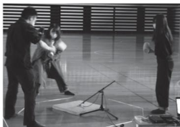
Fig.1: An EA method measurement conducted in-situ at the main arena of Gym-OU.
