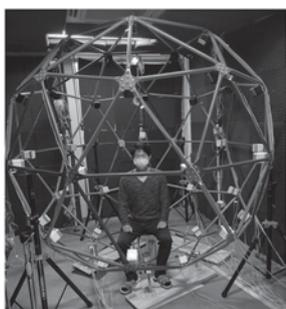
Fig. 1: 42ch geodesic dome type spherical loudspeaker array
