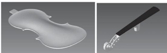
Fig.3: FE model for violin back plate and neck
