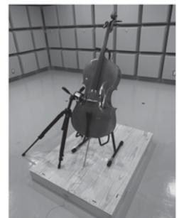
Fig.2: Measurement of cello using stage raiser.
