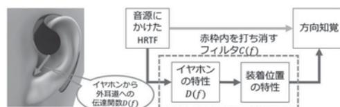
Fig.1: Overview of 3D sound reproduction using open-ear earphone.
