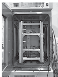
Fig. 1 Measurement device installed in a thermo-hygrostat.
