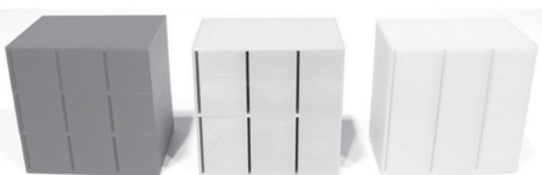
Fig.1: Samples of acoustic metasurface absorbers using microslits.
