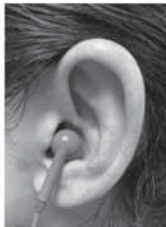
Fig.1: Cartilage conduction earphone for intercom Communication sound: Heard in both ears (clearly audible) Ambient sound: Heard in both ears (full perception of sound direction and distance)
