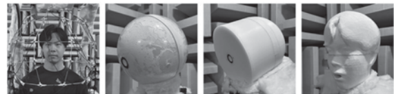
Fig.1: Speaker Fig.2: Sphere loudspeaker Fig.3: Front cylinder back hemisphere loudspeaker Fig.4: Dummy head loudspeaker
