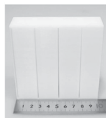
Fig.1: A sample of acoustic metasurface using microslits.
