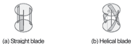
Fig.1: Shape of vertical axis wind turbine
