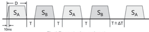
Fig.1 Perceptual experiment (perceiving the deviation \Delta T in the interval T between signals S_A and S_B )
