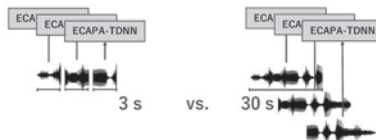
Fig.1: Dividing singing audio into shorter segments for pooling allows for more accurate representation of within-speaker variations
